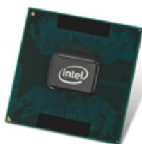
The Central Processing Unit – also known as the CPU or just processor – is the core and "brain" of the computer. This is where all of the essential calculations take place, and therefore it has a significant effect on almost everything you do on the computer.
